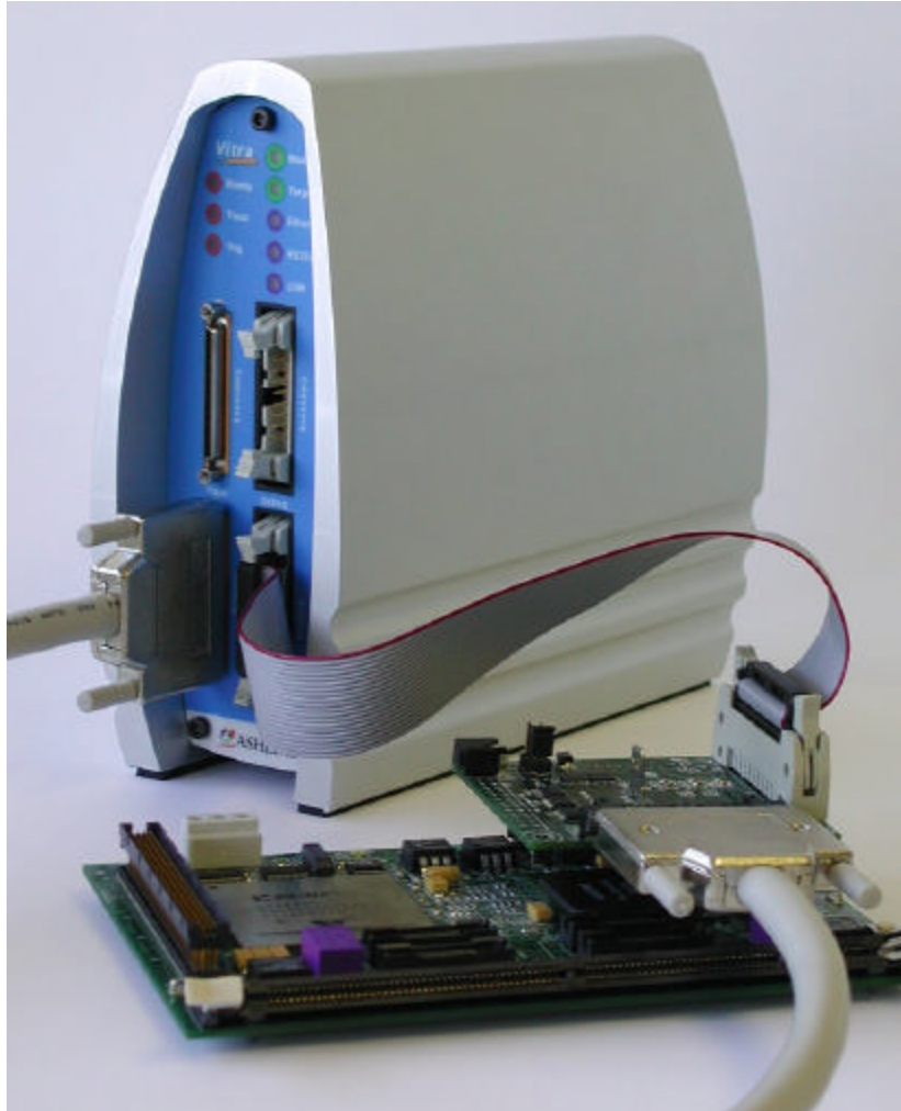
Ashling's Vitra Emulator includes full NEXUS Class 3 debugging, instruction trace and data read/write
